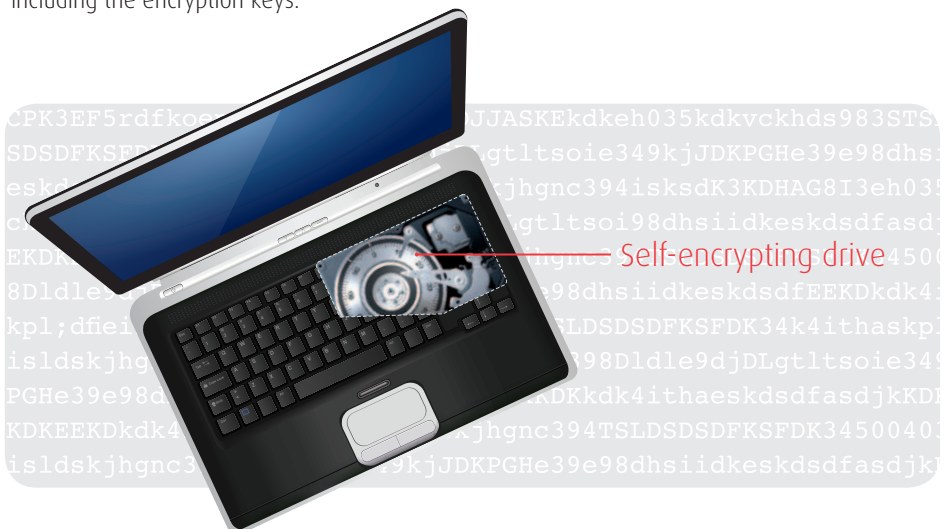
Fig 1. Computer manufacturers are building SEDs into new computers that comply with the OPAL specifications
